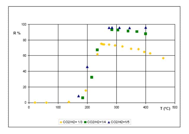
FIG. 1 –  $CH_4$  per cent yield plotted as a function of T at different  $CO_2/H_2$  ratios
